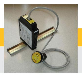
Connect **REMLIVE RL-24i** to the **OUTGOING** side of the Isolator / Circuit Breaker, making sure that the connections are electrically and mechanically sound and in accordance with current regulations for electrical installations. The **REMLIVE RL-24i** has embedded 50mA fuse link protection up stream of internal surge suppression. Dependent on the application it may be necessary to fit external fuse protection, typically 60mA rapid acting fuses.
